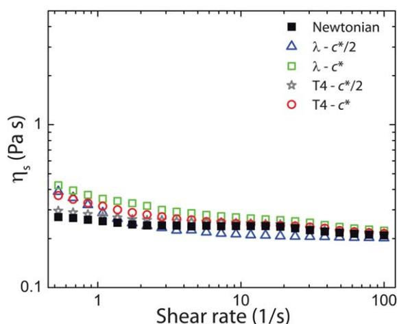
**Fig. 2** (Color online) Fluid rheological characterization. Shear viscosity *versus* shear strain rate for the Newtonian fluid and all DNA suspensions. DNA suspensions display slight shear thinning behavior with an average power law index of 0.80. The values of shear viscosities are nearly constant at a value of approximately 0.25 Pa s for all fluids beyond 1 s<sup>-1</sup>.
