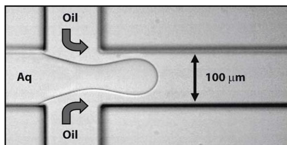
**Fig. 1** The experimental setup illustrating drop formation at the center of the cross-slot microchannel. The device is molded in PDMS and channel dimensions are  $100 \mu\text{m}$  wide and  $100 \mu\text{m}$  deep. The oil phase and the aqueous phase (Newtonian fluid and DNA suspensions) are injected into the device using low noise syringe pumps at inlets located 1 centimetre from the center of the cross-slot.
